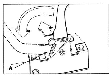
Figure 7: Adjust handlebars to "blower" position.
